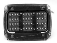
15. Test the tail lights, brake lights, and turn signals. If the turn signals do not flash you will need to upgrade your flasher. If you are replacing only the rear turn signals you should be able to use a heavy duty electronic flasher from your local parts store. If you are replacing both front and rear or do not have front bulbs you will need a no-load flasher, Dakota Digital part number LAT-NLF.
